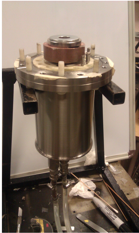
Figure 36. Experimental setup for Hall vacuum study with the sample mounted with thermal paste inside of a 1.0 T toroidal magnet placed on the copper cold head.
